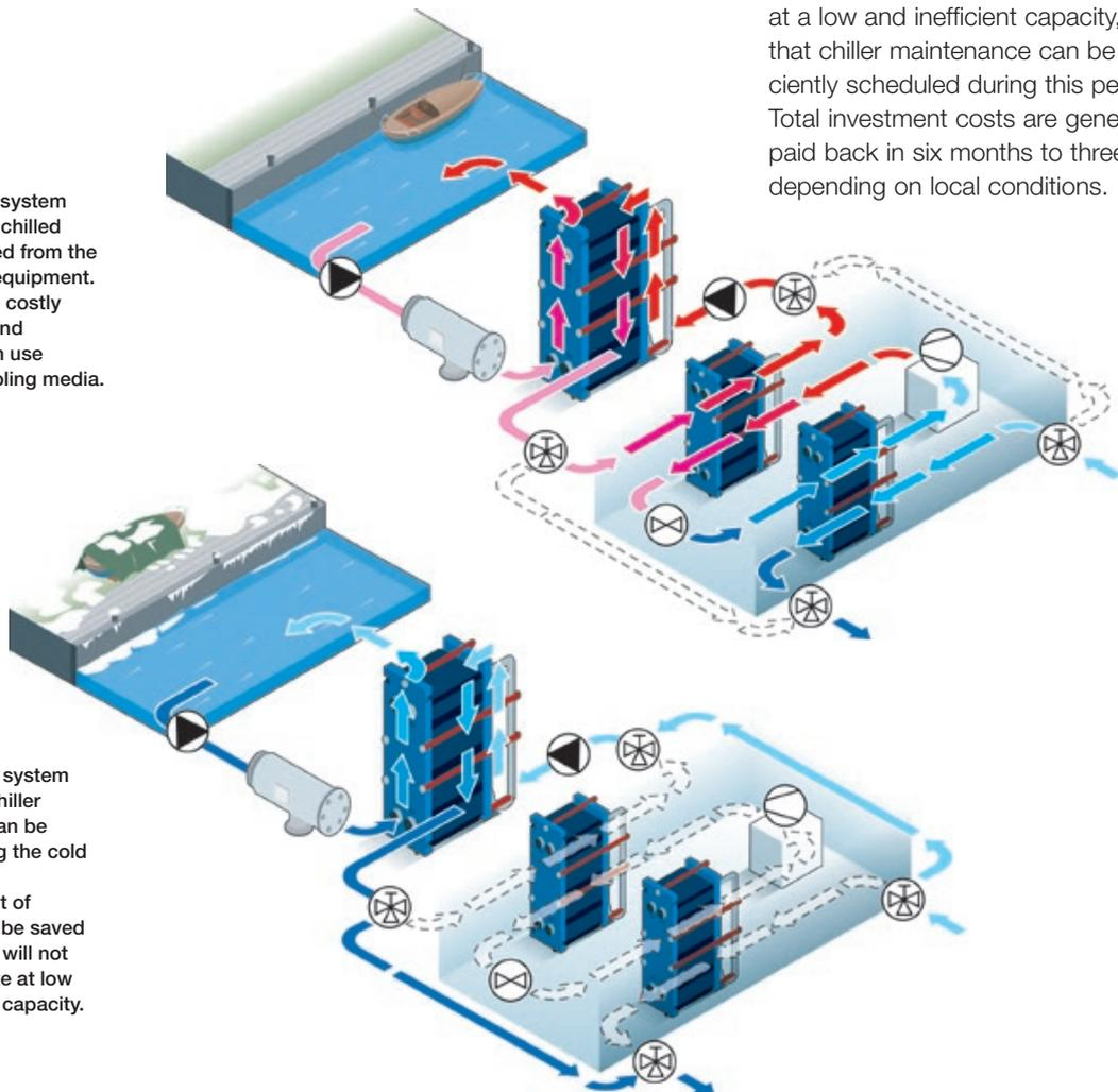
Chiller bypass system (winter). The chiller temperature can be reduced during the cold season. A large amount of electricity can be saved and the chiller will not have to operate at low and inefficient capacity.
