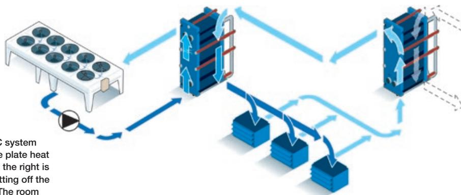
Reversible AC system (summer). The plate heat exchanger on the right is bypassed, cutting off the heat source. The room units are used as chillers.
