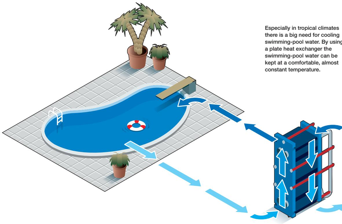
Especially in tropical climates there is a big need for cooling swimming-pool water. By using a plate heat exchanger the swimming-pool water can be kept at a comfortable, almost constant temperature.
