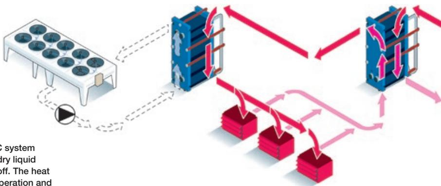
Reversible AC system (winter). The dry liquid cooler is cut off. The heat source is in operation and the room units are used as heat pumps.
