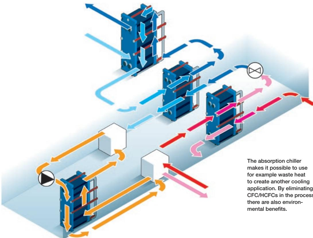
The absorption chiller makes it possible to use for example waste heat to create another cooling application. By eliminating CFC/HCFCs in the process, there are also environmental benefits.
