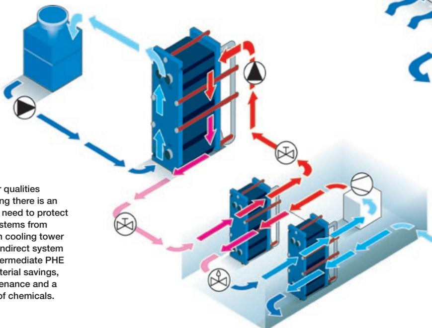
With water qualities deteriorating there is an increasing need to protect cooling systems from pollution in cooling tower water. An indirect system with an intermediate PHE means material savings, less maintenance and a minimum of chemicals.
