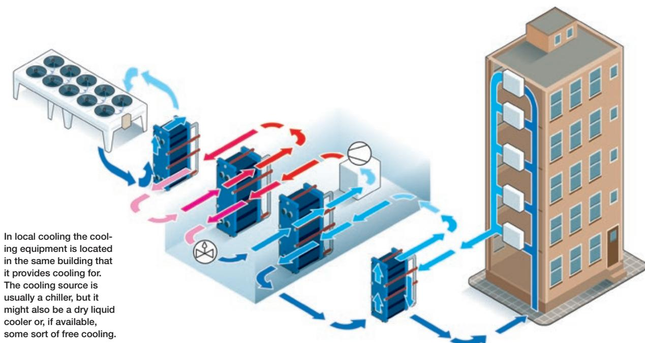
In local cooling the cooling equipment is located in the same building that it provides cooling for. The cooling source is usually a chiller, but it might also be a dry liquid cooler or, if available, some sort of free cooling.
