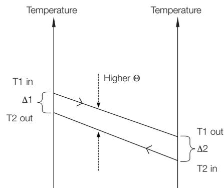
The diagram shows that small temperature differences result in high theta.
