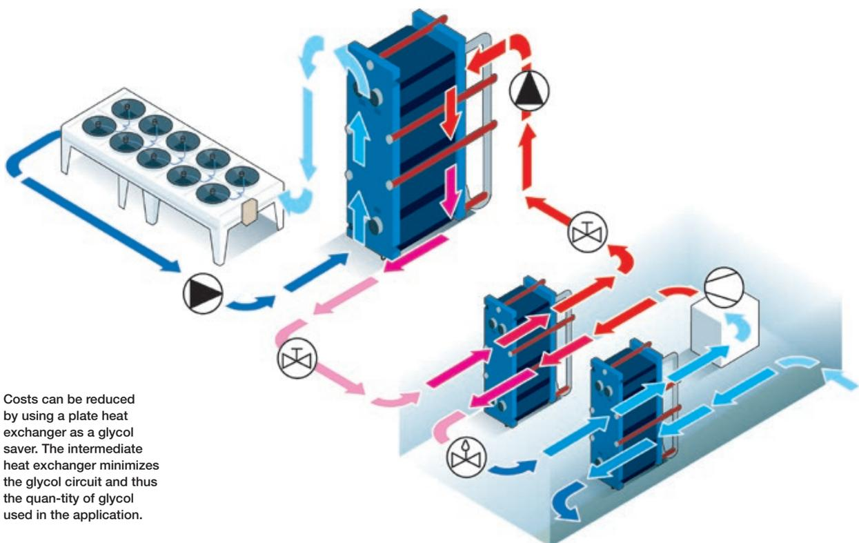
Costs can be reduced by using a plate heat exchanger as a glycol saver. The intermediate heat exchanger minimizes the glycol circuit and thus the quantity of glycol used in the application.
