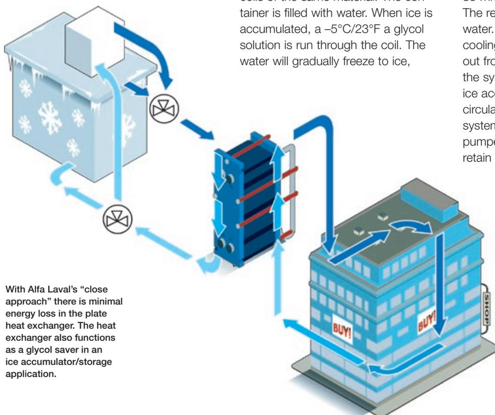
With Alfa Laval's "close approach" there is minimal energy loss in the plate heat exchanger. The heat exchanger also functions as a glycol saver in an ice accumulator/storage application.
