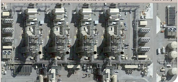
The Chuck Lenzie Generating Station, a combined cycle power plant near Las Vegas, Nevada was challenged to cool the closed loop auxiliary water while conserving make-up water based on allowed annual limitations of water availability.
