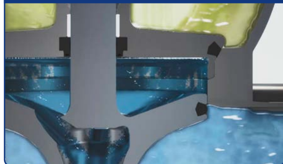
Figure 3. Seat push: The lower plug is pushed downwards thus cleaning the plug seal, seat and leakage chamber through CIP flow.
