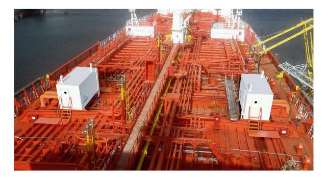
A new Alfa Laval PureBallast 3 Ex deckhouse solution has been validated for product tankers with Framo ballast pumps. The solution allows Alfa Laval PureBallast 3 Ex to be installed on deck – without any changes to the ballast pumping system on board.
